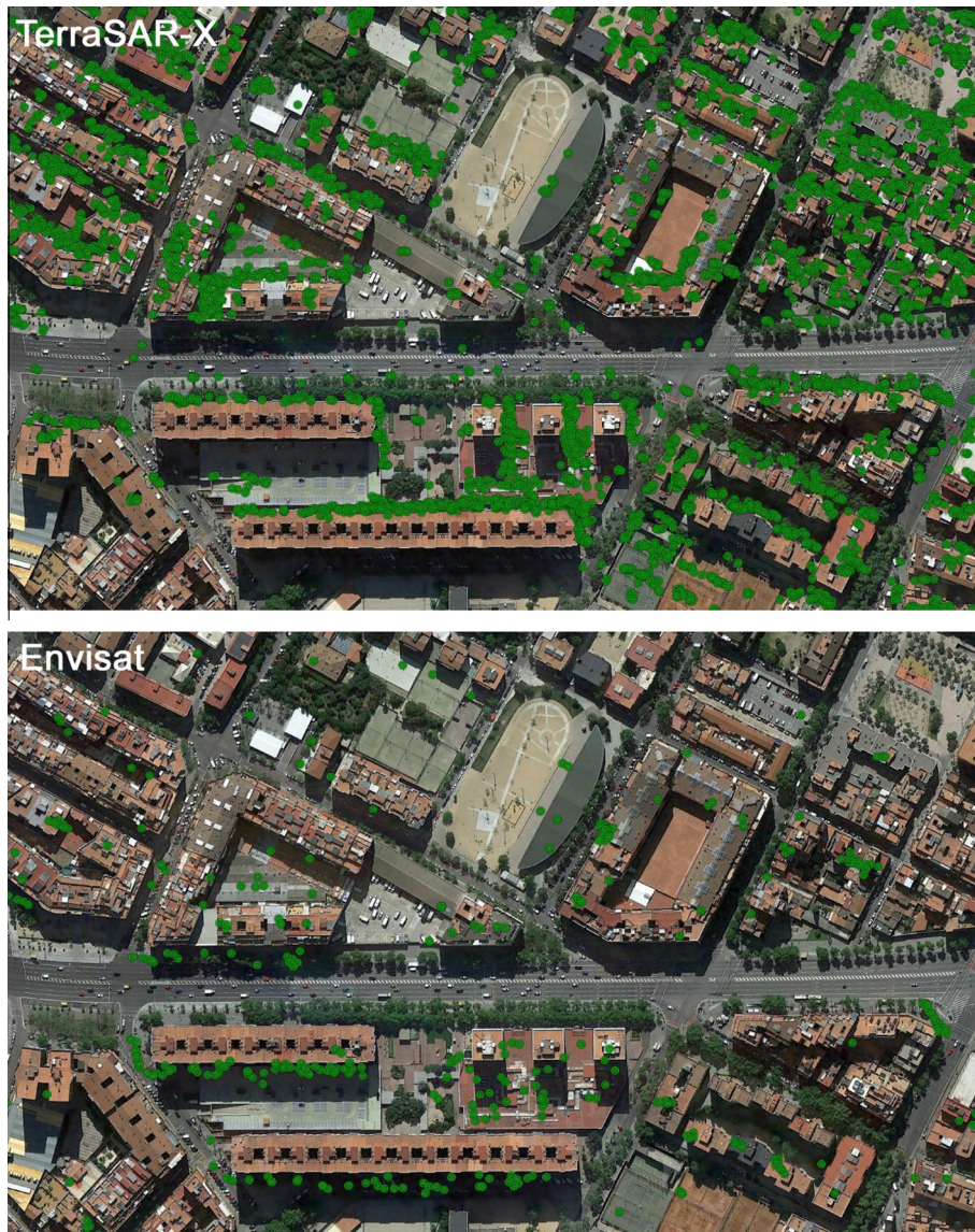
Fig. 3. Comparison of the Persistent Scatterer (PS) density achievable using C-band (Envisat) and X-band (TerraSAR-X) PSI.
